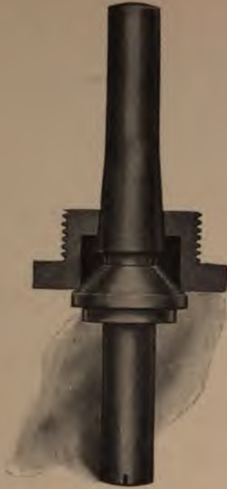
FIG. 48.—VALVE OF STEAM TRAP.
